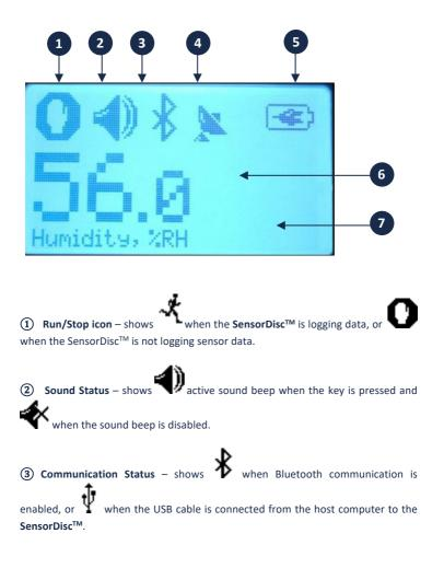
GPS Status – shows when the GPS is enabled, when locked to GPS satellites and provides valid positioning parameters.
